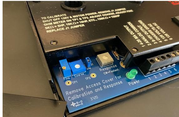
After making the correct power connections you should see a glowing green Power LED.
