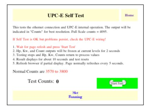
'Self Test' is used to verify correct network and UPC-E operation.
