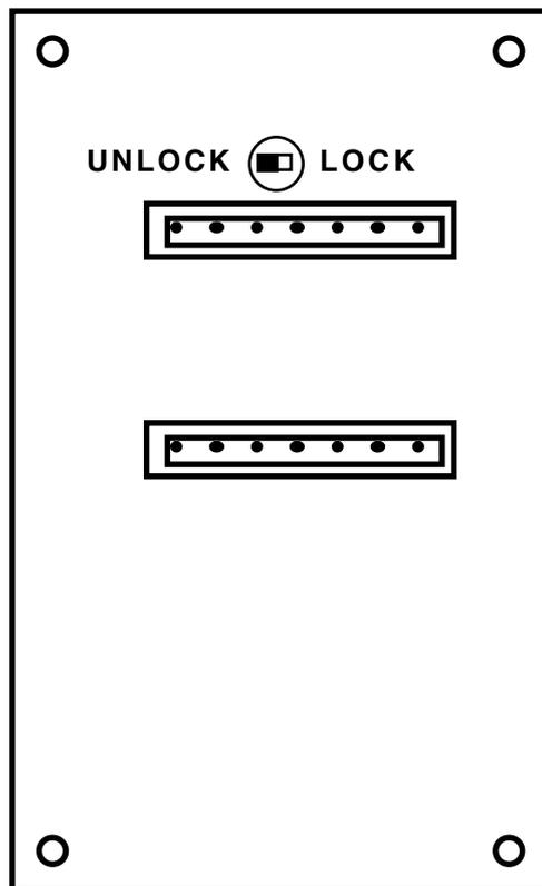
The Tamper Proof switch **LOCKS OR UNLOCKS** the front ENTER button. When the switch is to the **LEFT**, as shown, data can be entered or changed using the ENTER button on the front setup panel. When the switch is to the right, the ENTER switch is disabled and no data can be changed using the front setup panel.
