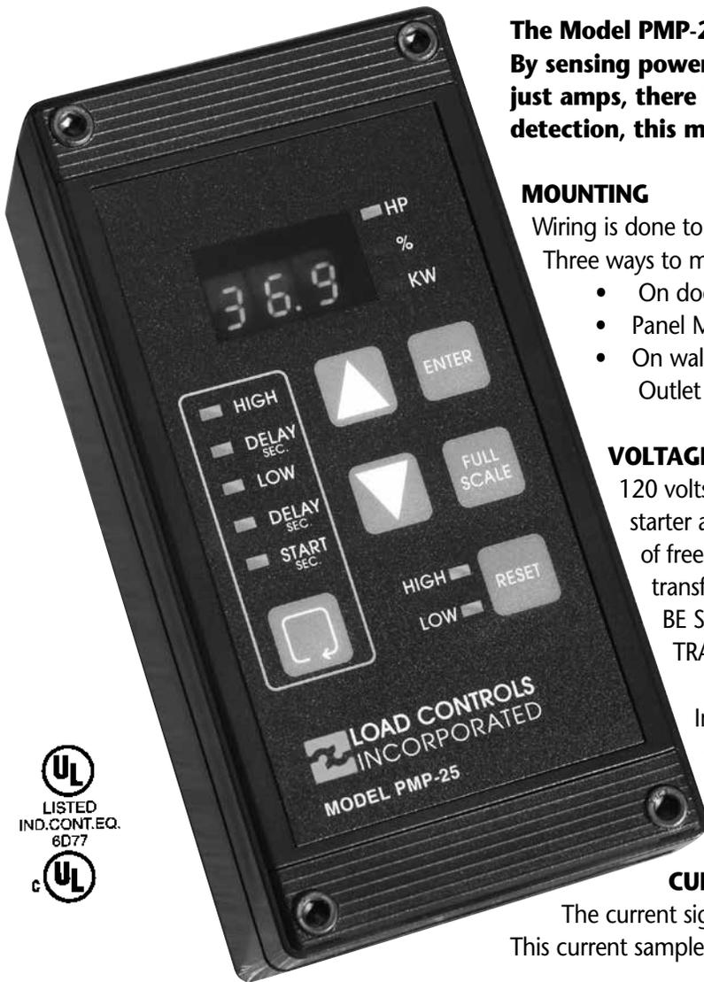
**The Model PMP-25 monitors the true power going to a motor. By sensing power (volts x amps x power factor) rather than just amps, there is much greater sensitivity. For loss of load detection, this means a 10X improvement in performance.**
