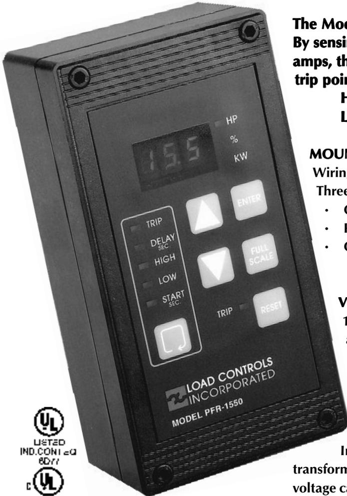
The Model PFR-1550 monitors the true power going to a motor. By sensing power (volts x amps x power factor) rather than just amps, there is much greater sensitivity. It has one adjustable trip point which can be either:
