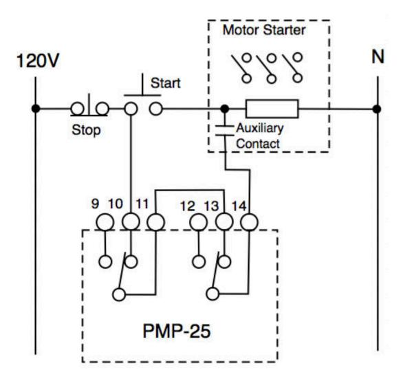
Reset - After a HIGH or LOW trip, the output contacts latch in the tripped condition and the trip indicator lights. The output contacts can only reset if the trip condition no longer exists or if the motor has been shut down and the START indicator is ON.
