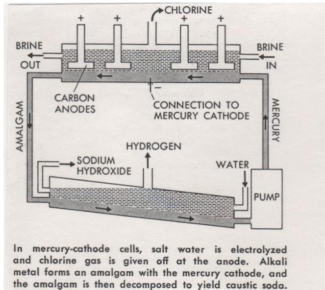
There are 60 pumps and occasionally a pump impeller will fall off or a pump will become jammed. If this happens the cast iron electrolysis tank becomes the cathode, and hydrogen is formed which is potentially explosive.
