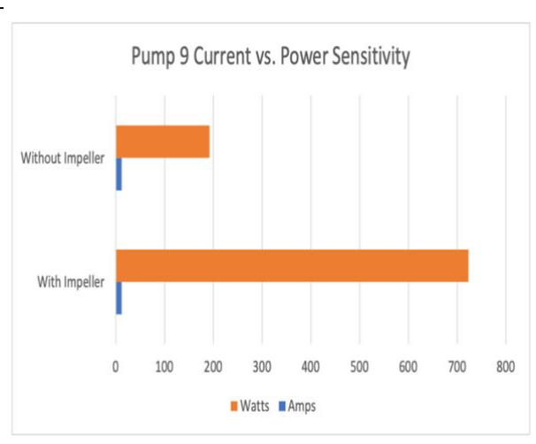
In an induction motor that is less than 50% loaded, the current changes very little with change in load. The thing that is changing is the power factor. Motor power is a much better measure of load since it works at both high and low loads and is linear.
