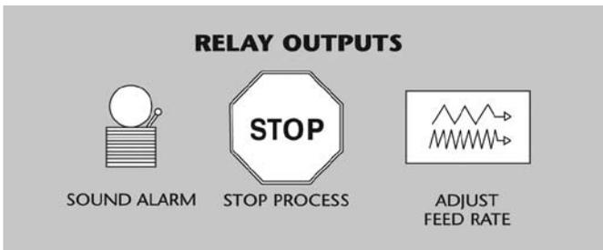
When the Set Point is reached the relay will switch (trip). Once it trips, it will latch in this position until it is reset (see RESET).
